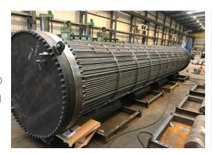
The use of anti-corrosive materials will increase the longevity of the equipment in service, saving the customer considerable money by reducing downtime and the need for carbon steel replacements.
