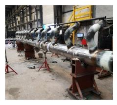
Unit Superheater Engineering facilitated the procurement of materials and machining from Western European suppliers. All manufacturing was completed at our main manufacturing facility in Swansea, South Wales. This included fabrication, pre-heating by ceramic braids, post weld heat treatment utilising our in-house gas fired furnace, in-house NDT and finally hydrostatic testing to 8000 psi.
